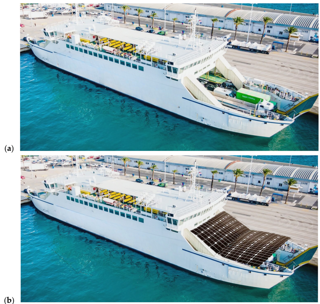
Figure 2. (a) The Ro-Ro ship in present state. (b) The Ro-Ro ship with designed solid carrier on the forward and aft deck open space parts.
