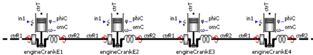
Figure 36. Sample structure of the multi-cylinder in-line engine with elastic crankshaft [80]
