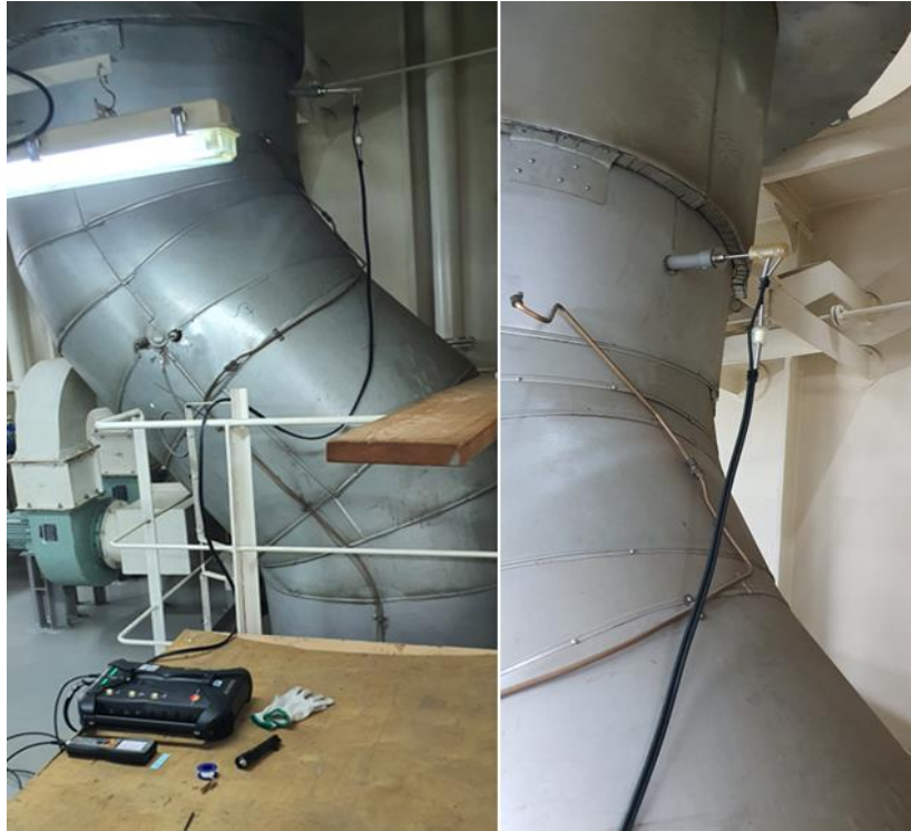
Figure 3.11 Position of the sampling probes during recording under real operating conditions.
