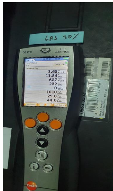
Figure 3.4. Example of an emission measurement while the engine is running on LNG
