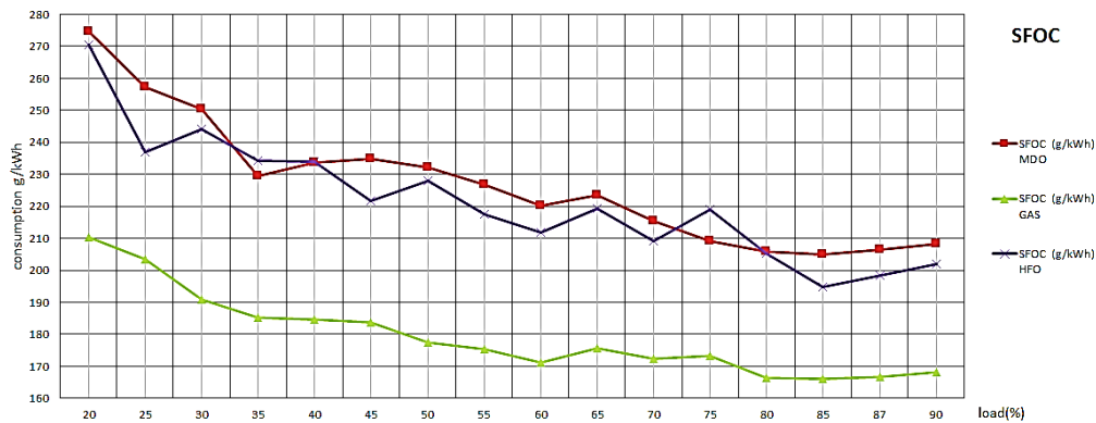
Figure 3.7 Fuel consumption data for three different types of fuel depending on the engine load
