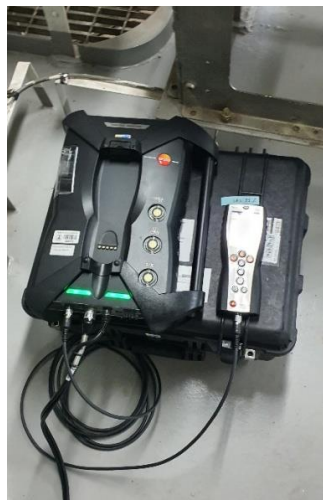
Figure 3.8 Exhaust gas analyzer “Testo 350 Maritime”, used for measurements on an LNG ship
