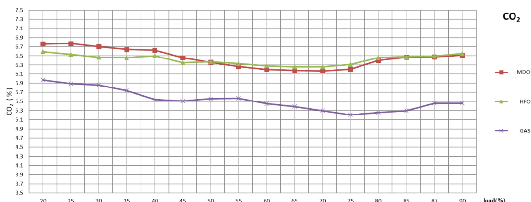
Figure 3.9 CO 2 emissions for three types of fuel depend on the engine load
