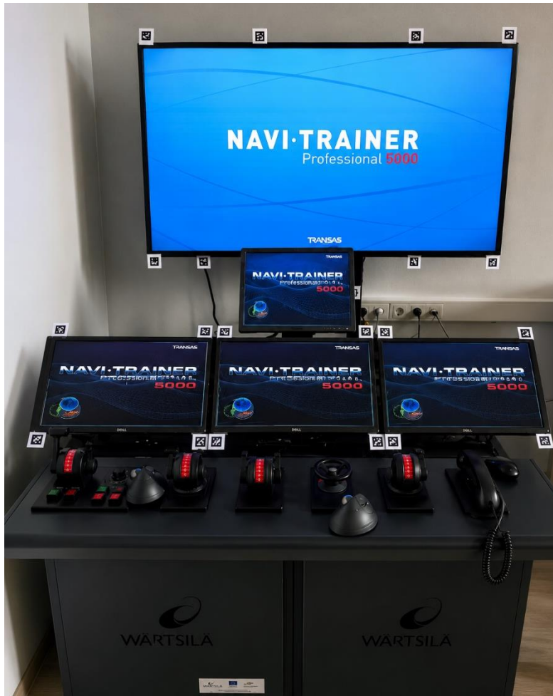
Figure 2.1 Wärtsilä Navigation simulator NTPRO 5000 (Navi-Trainer Professional 5000), “Tug console”
